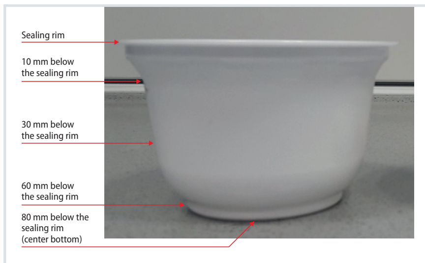
Fig. 1. Position of the wall thickness measurement in mm removed from the sealing rim
